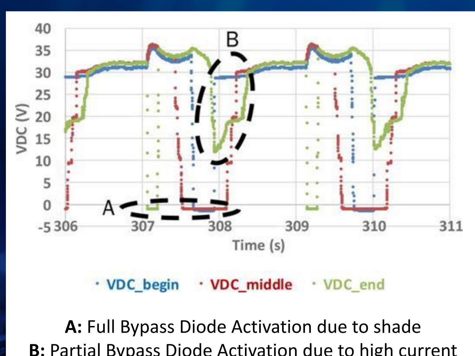
B: Partial Bypass Diode Activation due to high current \*In Field Data from TNO's study cited [1].
