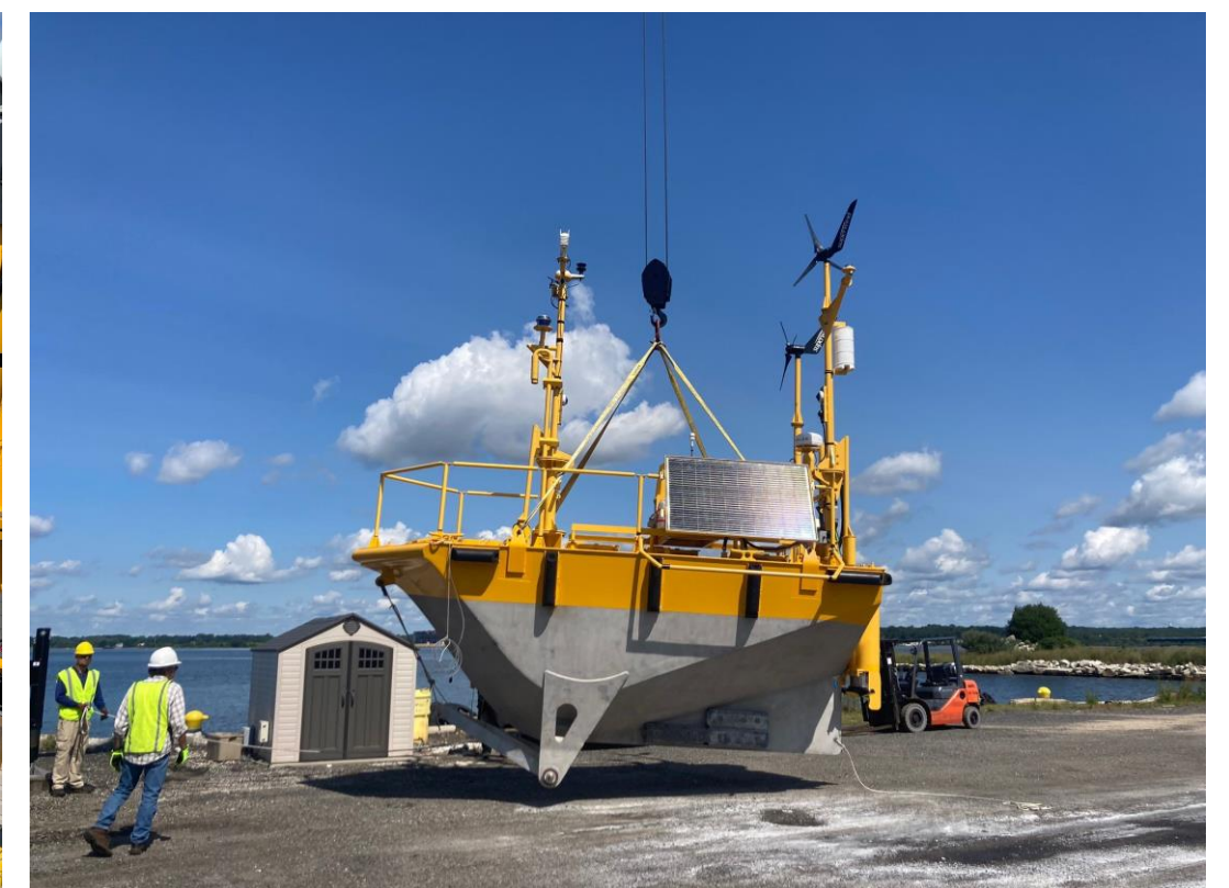
(Top) Schematic of the DOE test buoy with all key scientific sensors, power sources, and communication devices. (bottom) Buoy currently under testing at Fall River, MA. Additional Industry sensors added to the buoy for testing.
