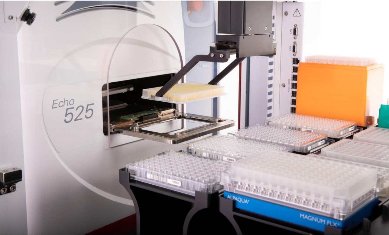
Biomek gripper loading an Echo Qualified 384-well Polypropylene Source Microplate onto the Echo source stage.
