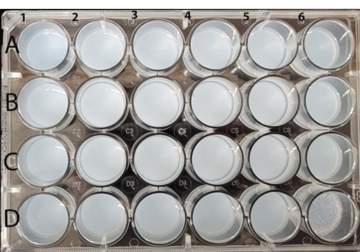
Figure 3: Encapsulation of amiCP biosensor. The reaction of SiNa and LUDOX with HCl allows for room-temperature encapsulation of bacteria.
