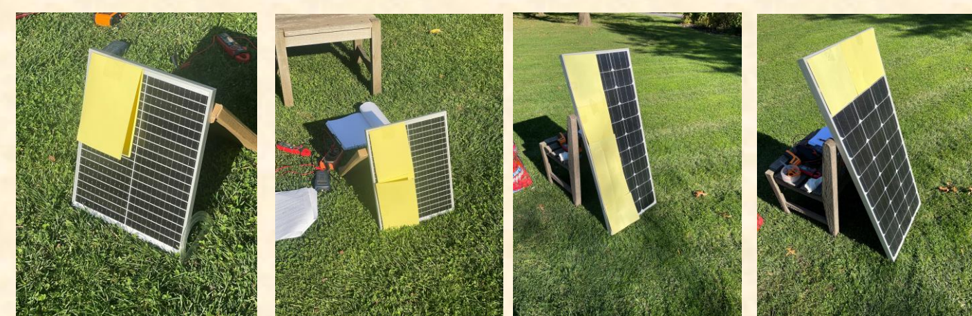
Fig.6: Shading the solar cells and comparing efficiencies.
