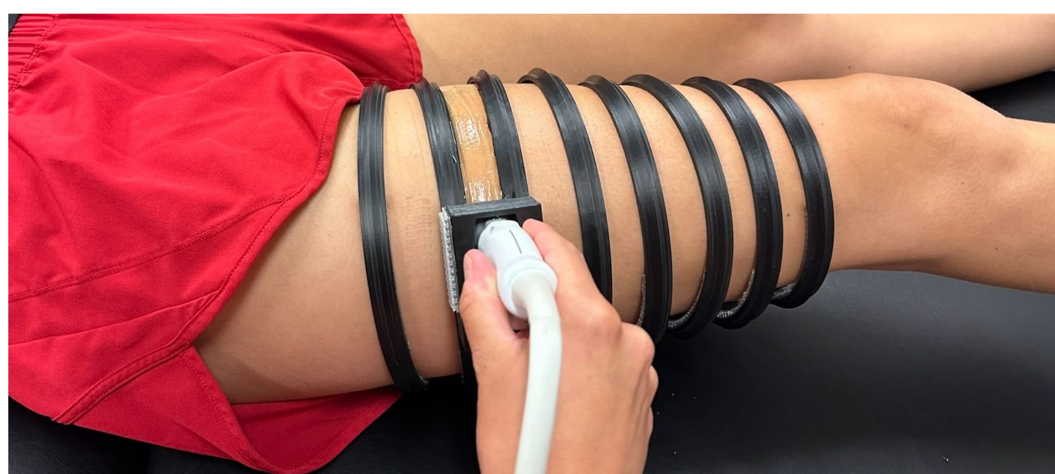
Figure 1. The 3D printed probe guide used to acquire ACSA scans. The cradle is used to control the pitch and yaw of the probe and is then placed on the customized tracks during cross sectional plane ultrasound scans
