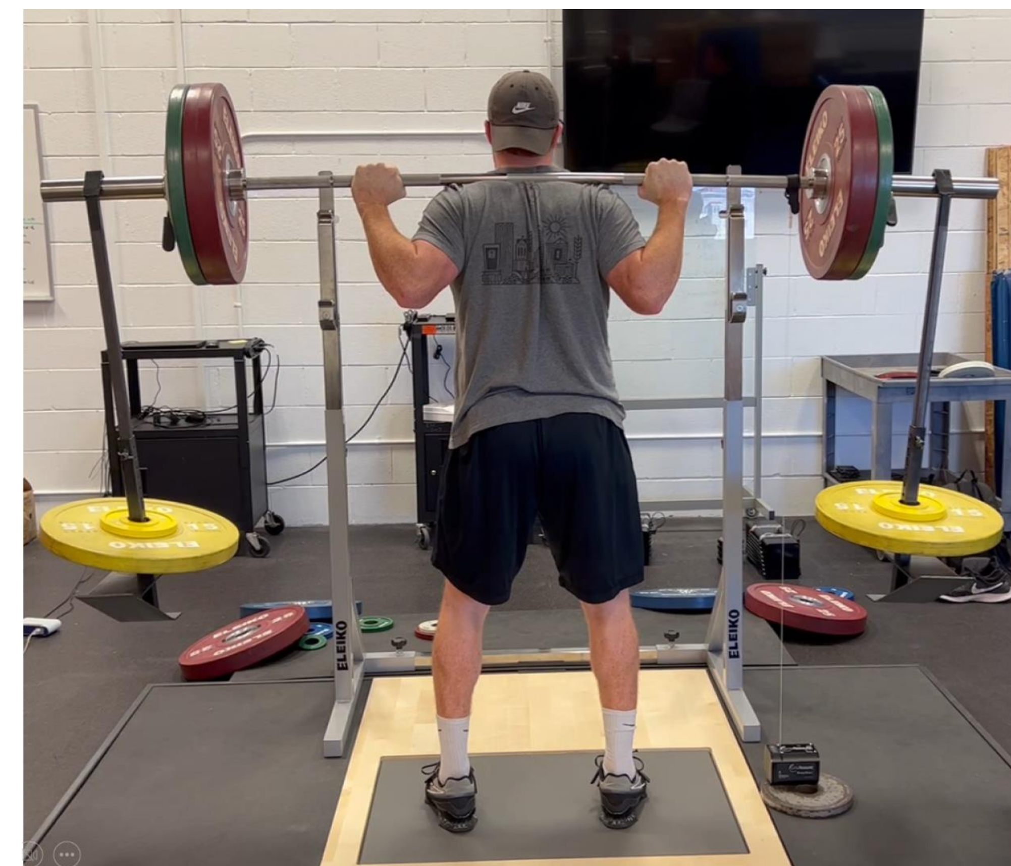
Figure 2. Starting position of the participant on the force platform with linear transducer attached and weight releasers on the barbell
