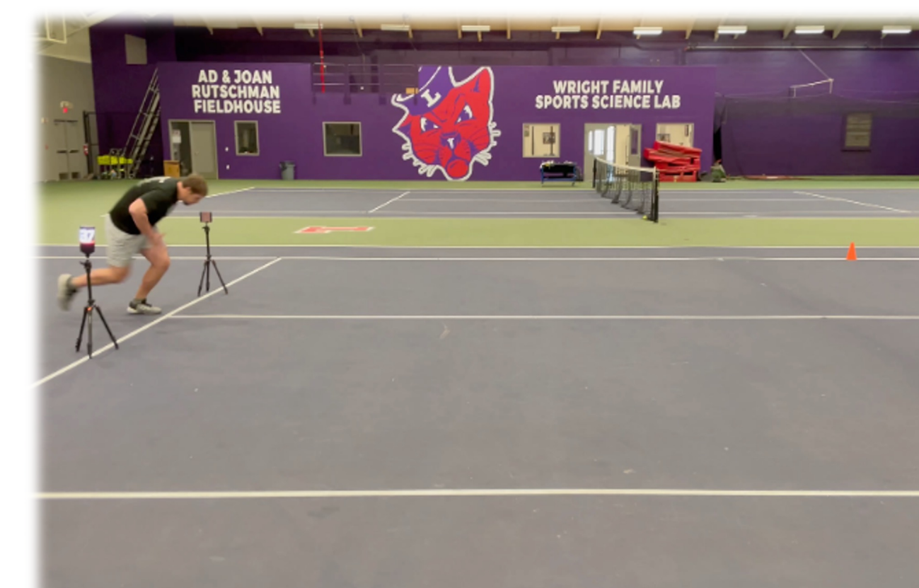
Figure 4: Photoelectrical laser timing system for 20-yard sprint and T-Test (VALD Performance, Queensland, Australia)
