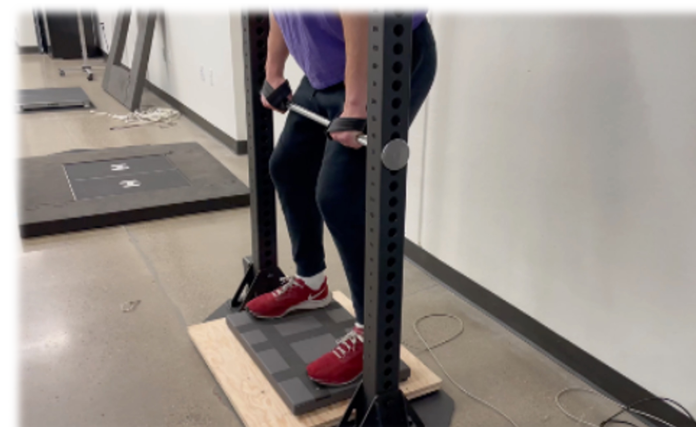
Figure 3: Isometric Mid Thigh Pull set-up with triaxial force plate system (Bertec, Columbus, OH; Hawkin Dynamics, Westbrook, MN; & Zeus Fitness, Vancouver, British Columbia, Canada)
