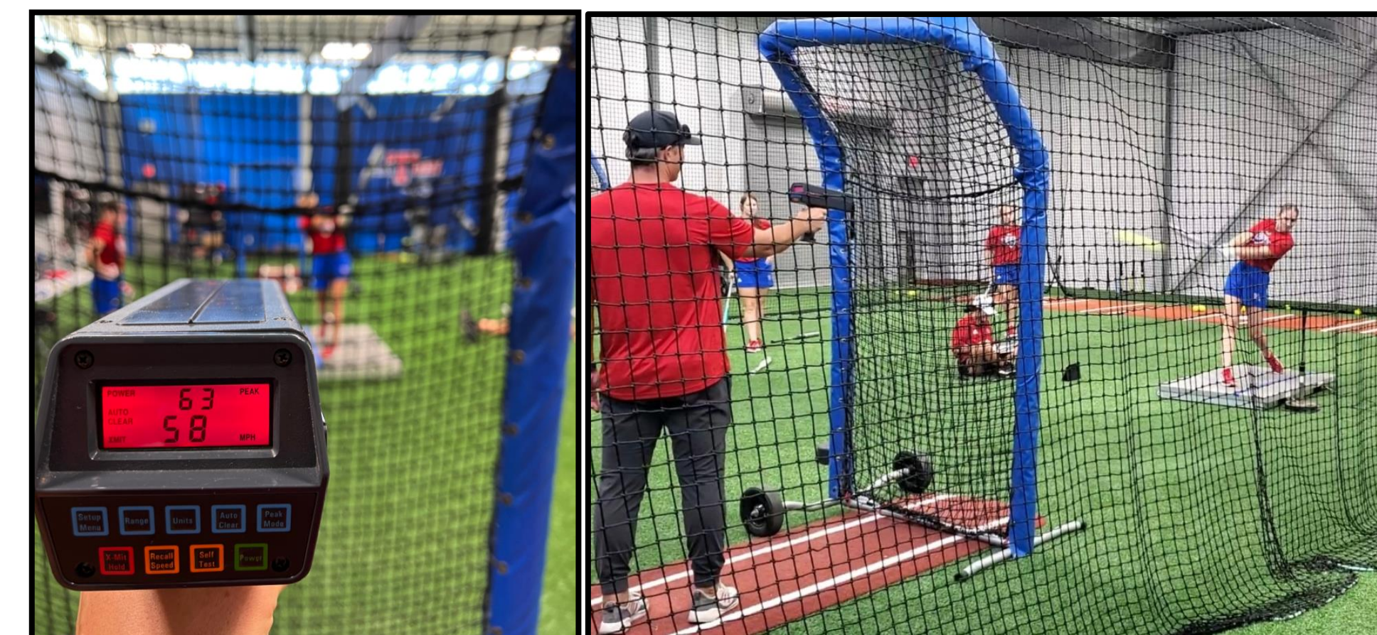
Figure 6. Stalker Pro radar gun used to measure exit velocity from behind screen.
