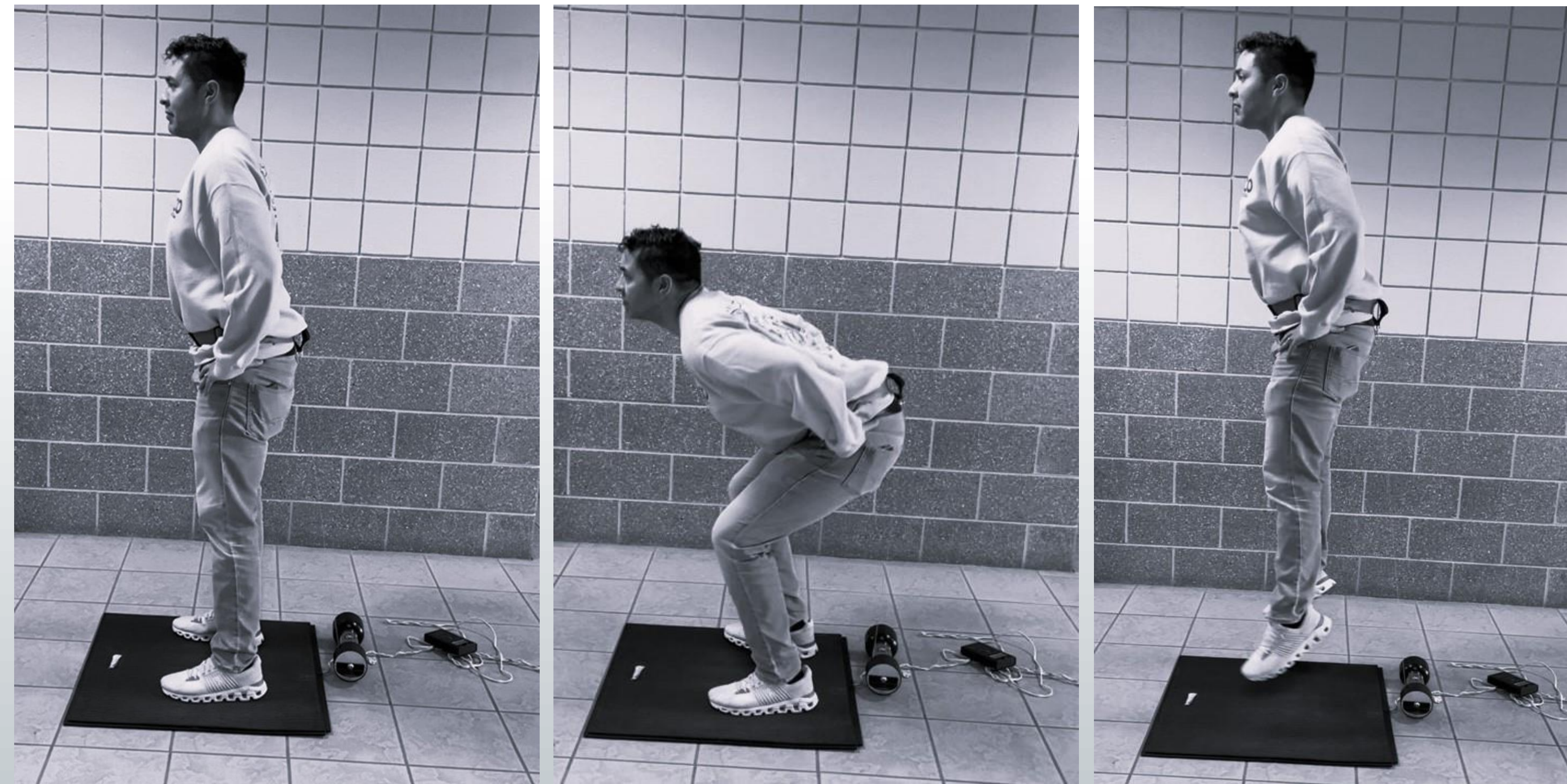
Figure 1. Includes pictures of the countermovement jump (CMJ) from start to finish. Athletes were instructed to keep hands on their hips the whole time, and were asked to jump as high as they could. The jumping mat measured vertical jump height, and the linear transducer measured average and peak power, as well as average and peak velocity.
