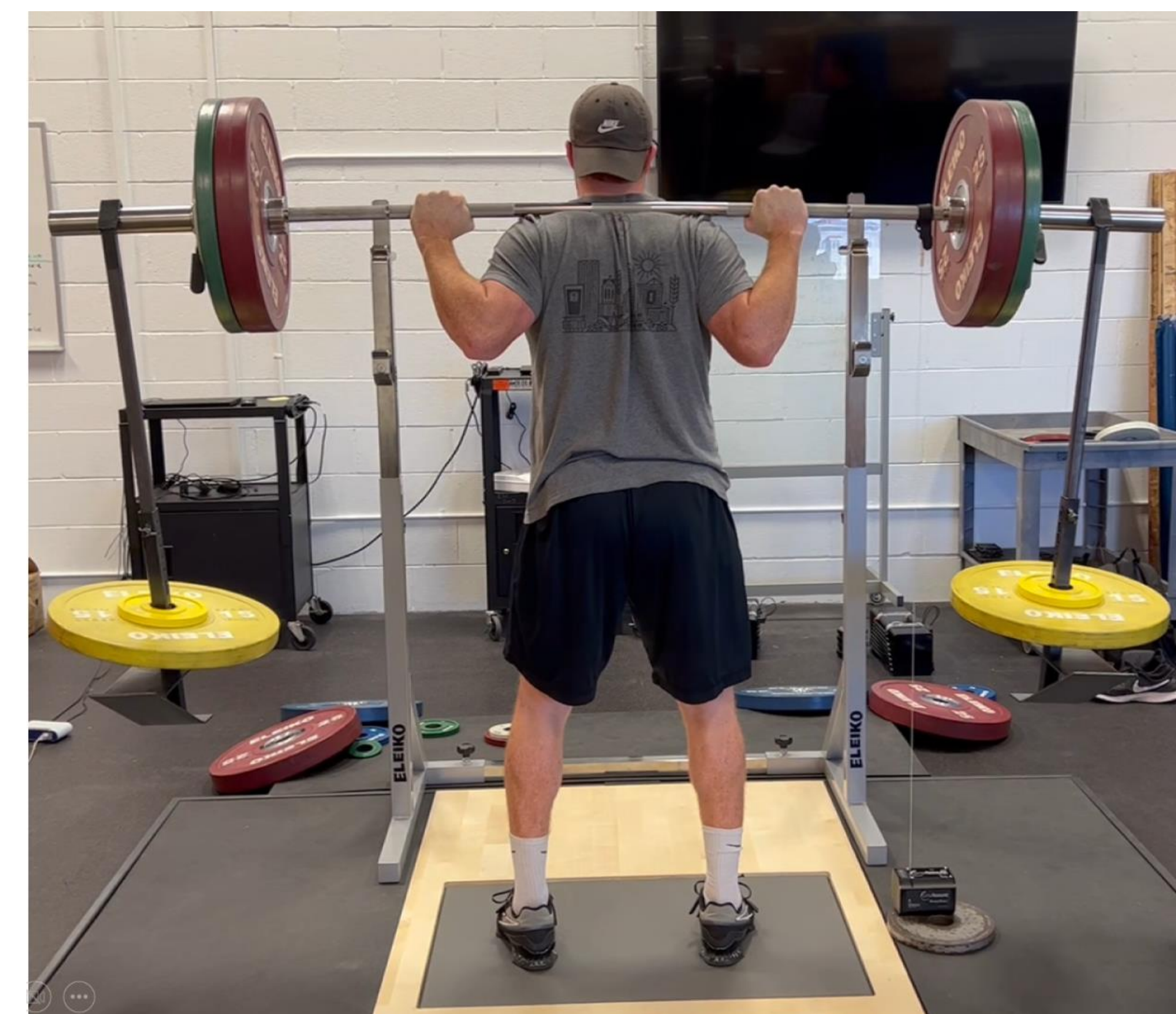
Figure 1. Starting position of the participant on the force platform with weight releasers on the barbell.
