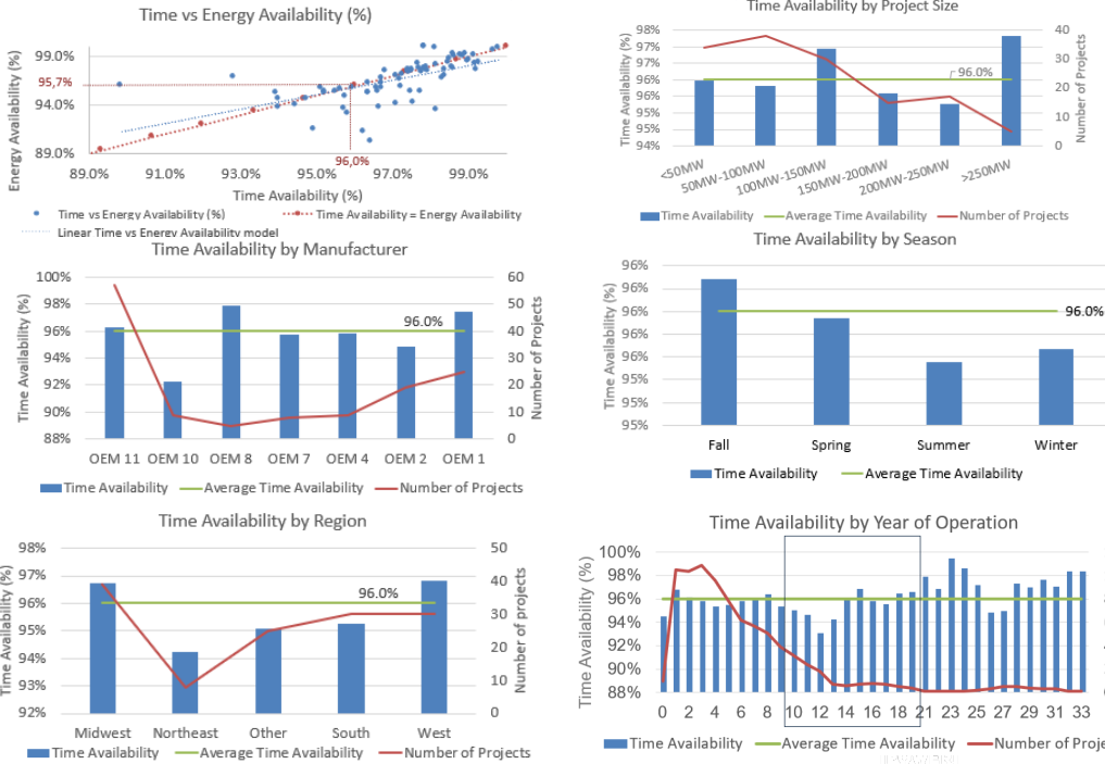
Figure 2: Time vs Energy, Availability by size, OEM, season, region and year of operation (only projects with pre-2006 COD)
