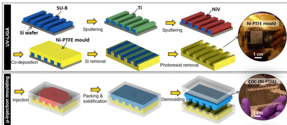
Fig. 2. The fabrication process of Ni-PTFE nanocomposite mold, and the electroformed Ni-PTFE mold with the produced COC chip from micro injection molding process.
