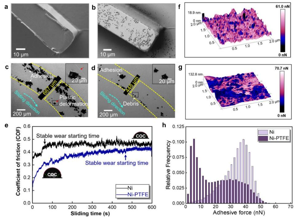
Fig. 5. Surface morphology of the (a) Ni mold and (b) Ni-PTFE mold after injection molding. Wear morphologies on the (c) Ni and (d) Ni-PTFE. (e) COF of two molds against the COC pin. Adhesive force mapping overlaid with surface topography of (f) Ni and (g) Ni-PTFE detected by AFM. (h) The histograms of the adhesive forces distribution.
