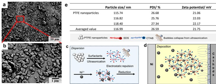
Fig. 1. SEM images of PTFE nano-fillers as powder (a & b); the mechanism of nanoparticle dispersion and co-deposition (c & d); the particle size, PDI and zeta potential of PTFE nanoparticles in the electrolyte (e).
