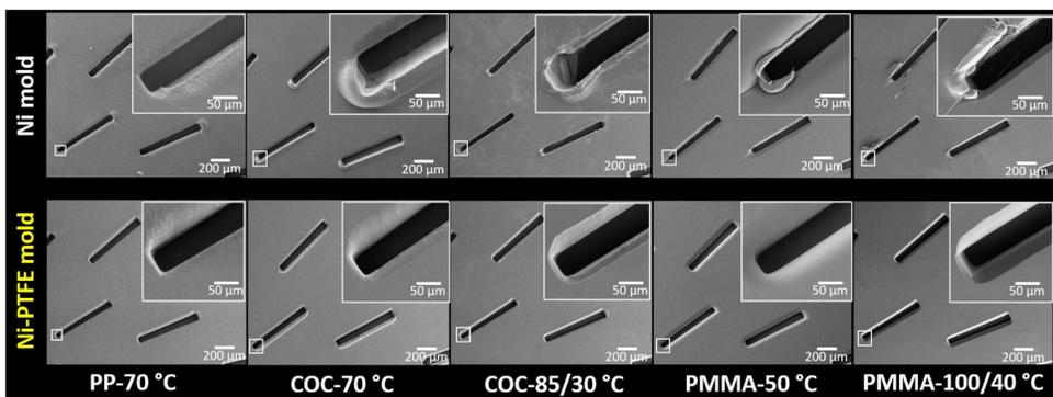
Fig. 3. Surface morphology of injection molded PP, COC and PMMA under different mold temperatures.
