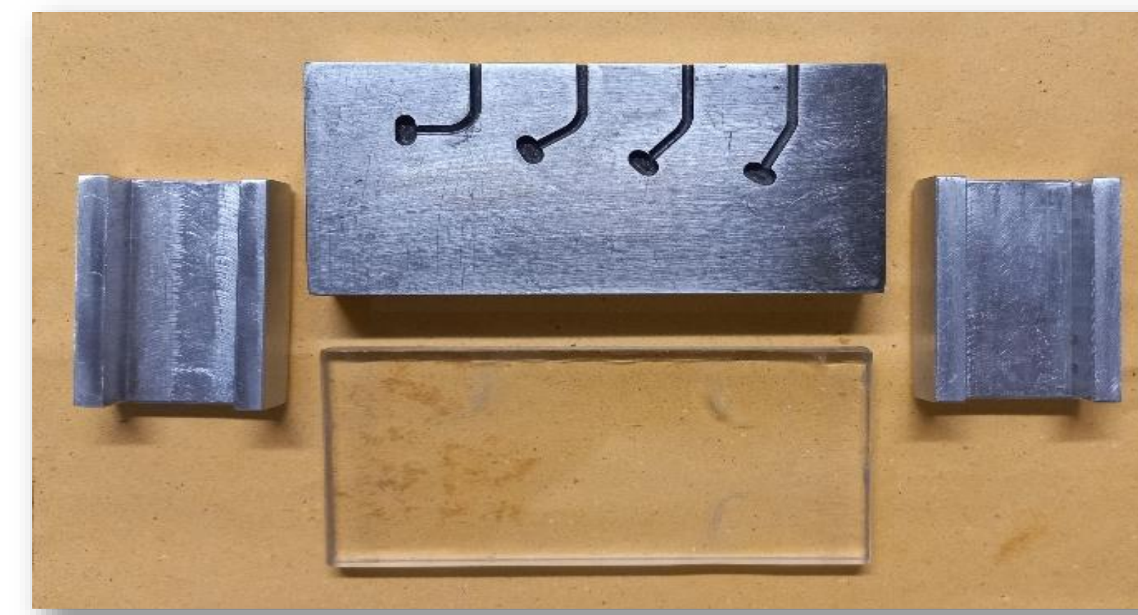
Fig. 2. Simulated root canals device.
