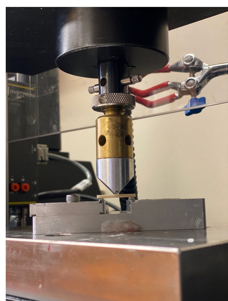
Figure 1. Apparatus used for testing flexural strength of Glass Ionomer rods.
