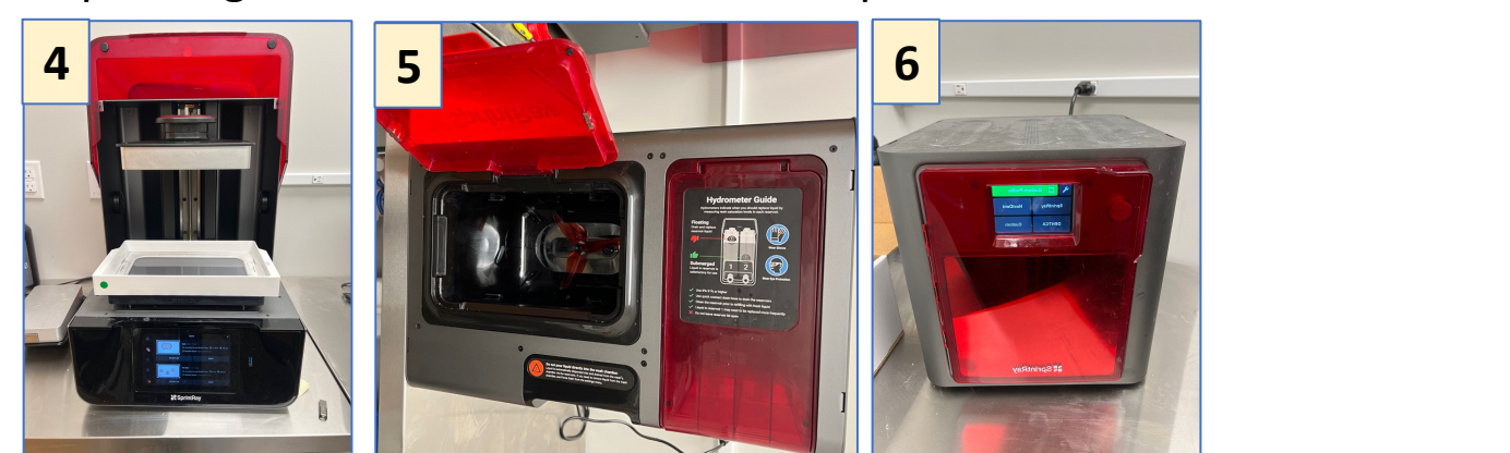
Figure 4: 3D Resin Printer Figure 5: 3D Resin Ethanol Washer Figure 6: 3D Resin Oven
