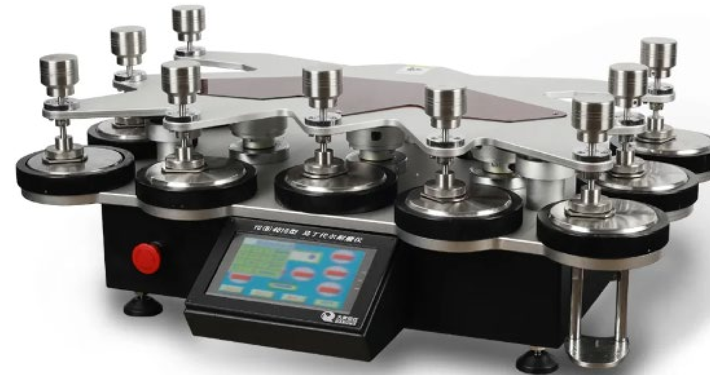
Figure 2: Martin Dale Fraying test to simulate 175,000 rub cycles.
