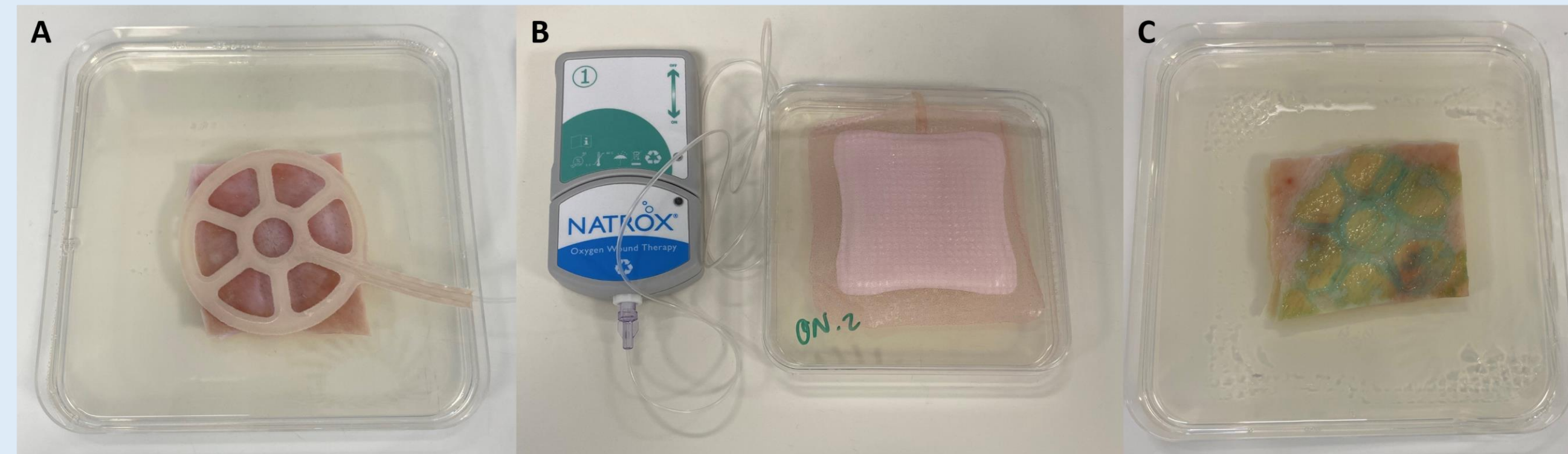
Figure 1. A) cTOT device placed onto inoculated porcine skin, B) skin & cTOT device covered with 10 cm x 10 cm semi-permeable dressing, C) Final assay result following 24 hour humidified incubation at 37 °C ± 2 °C.
