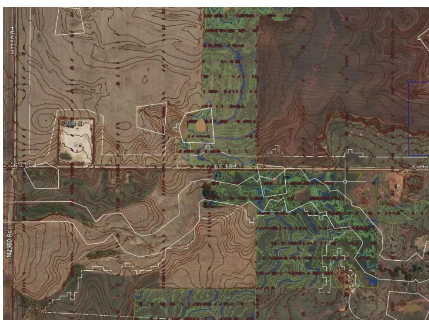
LiDAR data as topographic lines (dark brown) for an Invenergy project, alongside buffers of wetland and waterways mapped by the National Wetland Inventory and National Hydrography Data (white lines).
